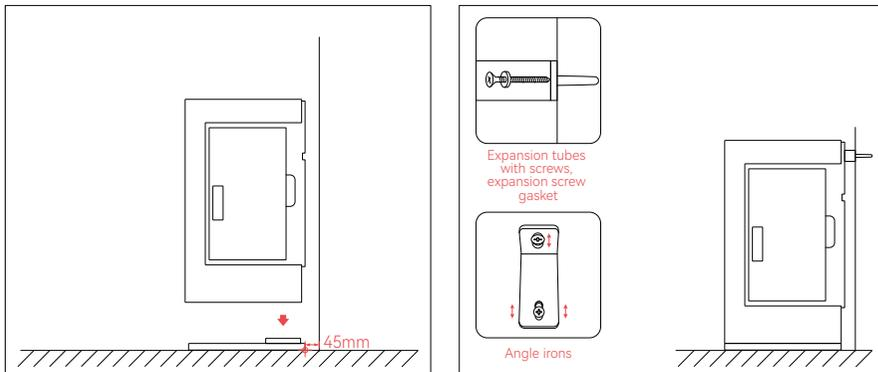
Mark the position at 45mm from the wall, place the base parallel to the wall (the waterproof sleeve for the connector is already installed on the base, do not remove it). Align the bottom connection port of the inverter with the anti-falling slot on the base and place it on the base.
