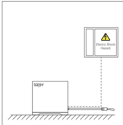
Measure the distance between the product and the power distribution box using the tape, and select a ground wire of appropriate length.
