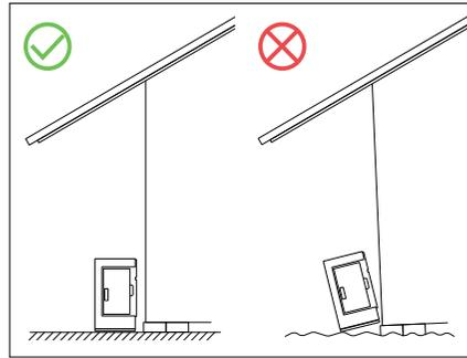
For stability, the product should be installed on solid and flat ground, with the wall being perpendicular to the ground.
