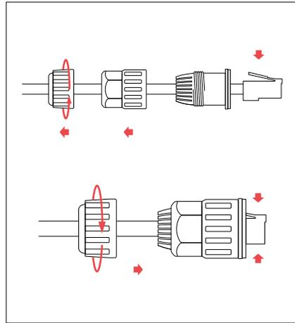
Insert it into the waterproof rubber sleeve and push the rear terminal forward. Press the crystal head and tighten the end of the terminal.
