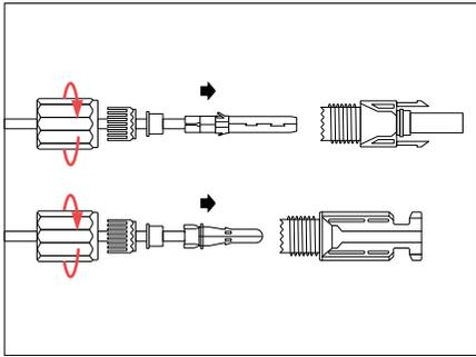
Insert the terminal into the wiring slot, until you hear the sound indicating a proper connection. Tighten the end of the terminal. Ensure the cable and terminals are connected securely.
