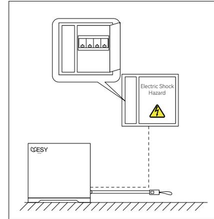
Turn off the circuit breaker of the power grid. Measure the distance to the power distribution box using the tape, and select a cable of appropriate length. Secure the terminal according to the load connection steps in 5.5.
