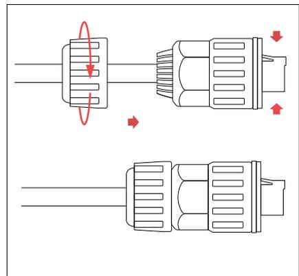
Tighten the end of the terminal and check if the connection is secure.
