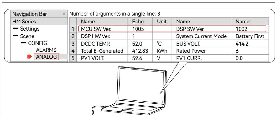
**View Firmware Version:** On the ANALOG page of the upper computer, check the MCU SW Ver. and DSP SW Ver. to obtain Firmware Version information.
