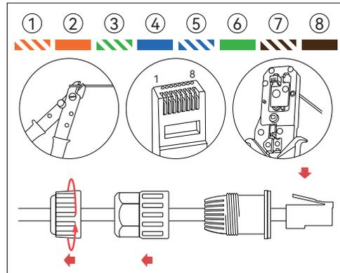
Use a wire stripper to separate the Ethernet cable and pass the wires through the corresponding parts in the sequence shown in the diagram. Press the wires into the crystal head in the order of colors 1 to 8 using an Ethernet crimper. After firmly securing the crystal head on the terminal, insert it into the terminal head.
