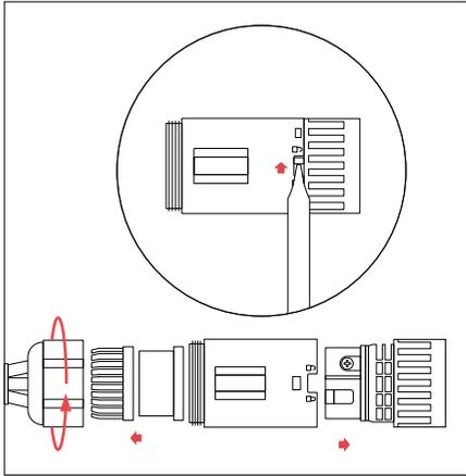
Twist the terminal at the back end, open the rear cover, and separate the waterproof rubber ring. Use a screwdriver to open the other end of the terminal's fuse, and then pull out the front end of the terminal.
