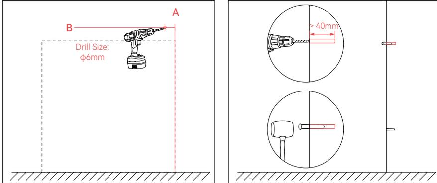
Use a  $\phi 6\text{mm}$  drill bit to drill holes at the marked positions.
