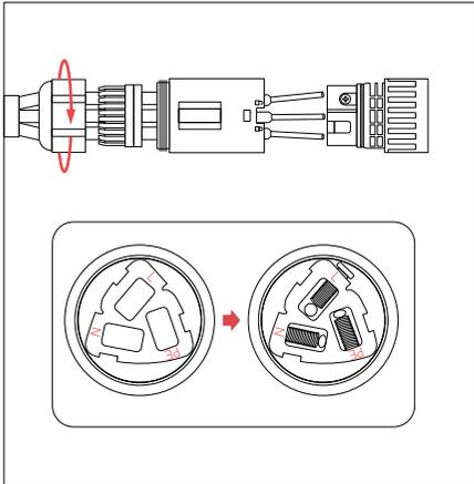
Connect the cables to the terminals according to the sequence shown in the diagram and secure them using screws. Tighten each terminal in sequence from front to back.
