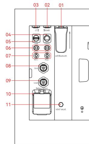
Lateral marks on the HM Series Inverter chassis
