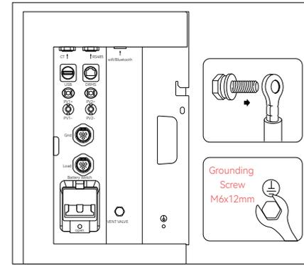
Fasten the ground wire terminal to the right radiator of the equipment using the ground wire screw ( $\phi$ 6mm), and ensure that the other end of the wire is properly grounded with the grounding impedance of 0.1 $\Omega$  or less.
