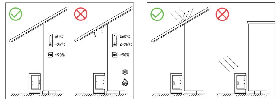
The ambient temperature should be  $-25^{\circ}\text{C}$  to  $60^{\circ}\text{C}$  and the relative humidity should be 0% to 90% (no condensation).
