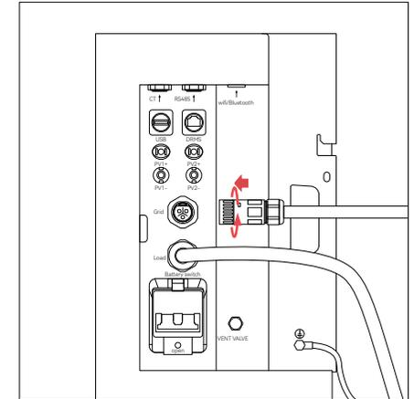
Insert the terminal into the Grid interface, and rotate the tail part of the terminal until it is secured, and check.
