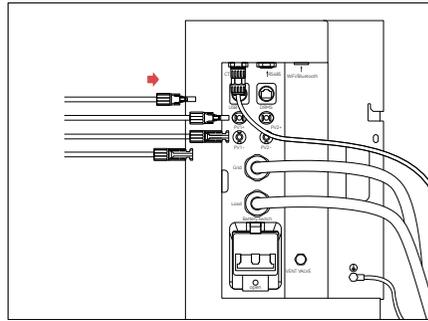
Determine the polarity of the PV input terminal of the equipment and that of the machine. Connect the PV input cable to the equipment. Ensure the cables are connected properly.
