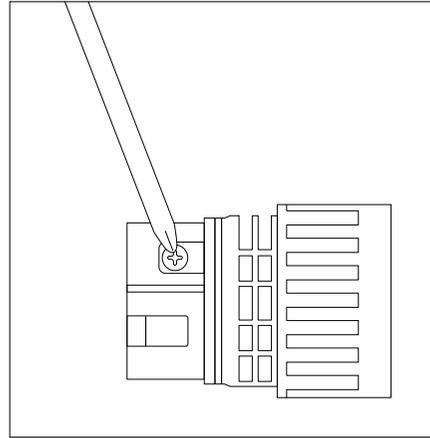
Use the Phillips screwdriver to remove the screws from the front terminal. Standard Torque: 0.8 Nm.
