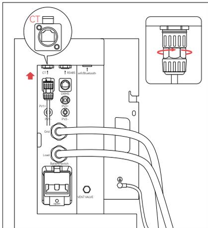
Insert the terminal into the CT interface, tighten the terminal and ensure the cable is connected securely.
