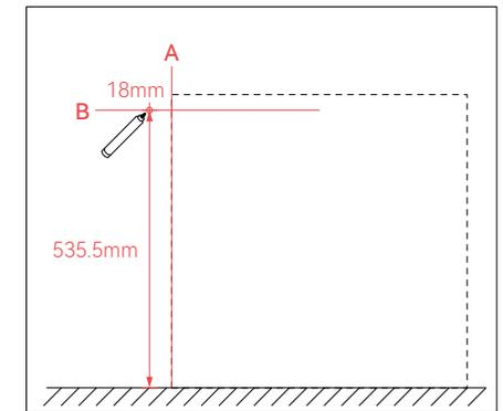
Select the left boundary of the chosen equipment and mark it. Fix the Y-axis of the level to the left side of the equipment and draw reference line A. The reference line should be perpendicular to the ground.
