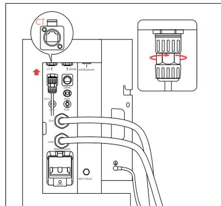
Connect the Ethernet cable with waterproof connectors to the RS485 interface on the inverter casing.
