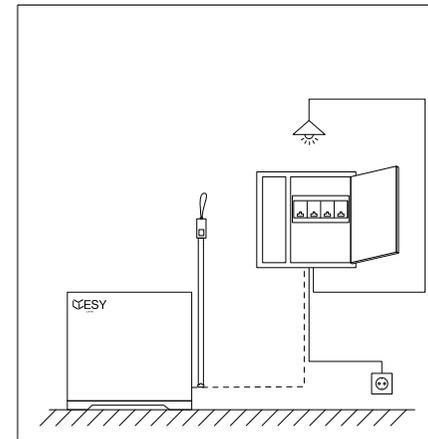
Measure the distance between the product and the power distribution box or load terminal using the tape, and select a cable of the appropriate length.
