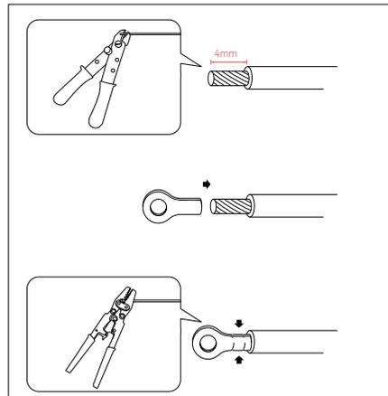
Strip the ground wire insulation by 4 mm using the stripping pliers, install the ground wire terminal, and press it tightly with crimping pliers.
