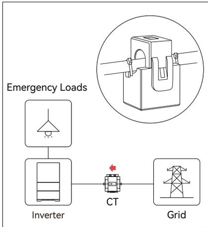
Place the CT on the grid side, with the arrow on the CT ("→") pointing towards the inverter and household loads.
