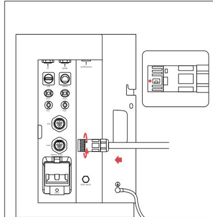
Plug the terminal into the Load interface, and press the buckle as shown. Then check all wiring for firmness.
