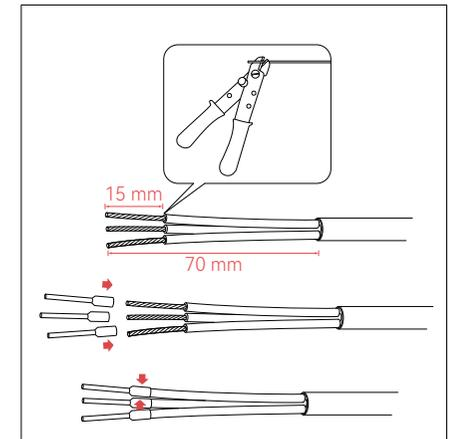
Strip the cable sheath by 70 mm and core insulation by 15 mm using the stripping pliers. (Note: Use ferrule crimping pliers to crimp an insulated cord end terminal 6 mm<sup>2</sup> onto the cable.)
