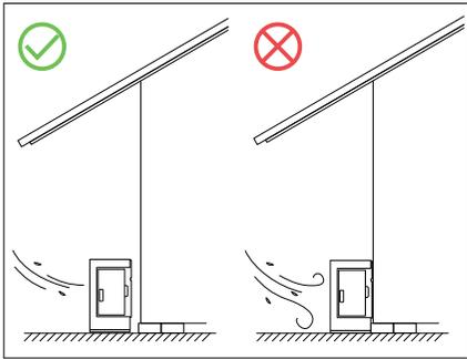
This product is self-cooled. To ensure proper heat dissipation, please install it in a well-ventilated place.
